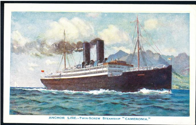
To begin with, earlier this ship was termed as TSS and now as SS Cameronia. TSS references that this ship was a "Twin Screw Steamship" while SS would simply refer to the ship as a "Steam Ship." Both terms are forms of advertising and descriptors of the ship. SS would refer to a reliable service since power was provided by a steam engine instead of wind (sail), while TSS would provide an impression of a faster, better form of travel using two propellers.
